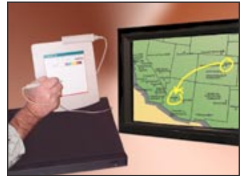
The Pointmaker PVI-44 color video marker main unit (left) with digitizing tablet.
